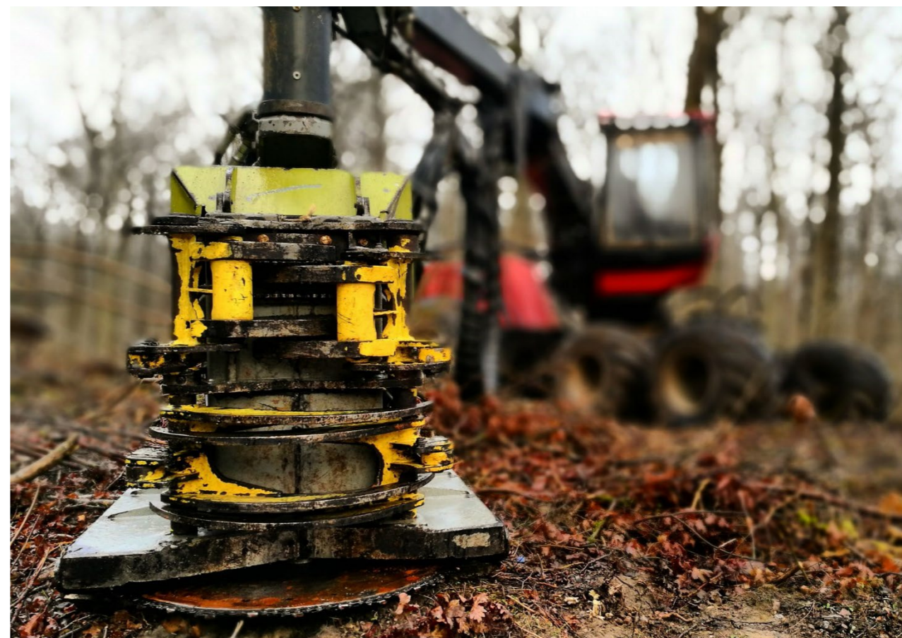
Pic.10: Forestry harvester machine equipped with a tree shear head
